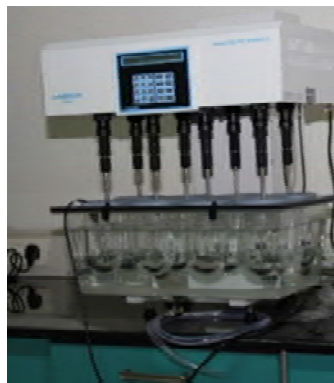
Dissolution test apparatus for carrying out tests per the Indian Pharmacopoeia method 2.5.2 and other compendia.
