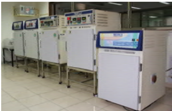
Equipment for accelerated stability and photostability studies as per Appendix IX of The Drugs and Cosmetics Rules, 1945/2016 for assigning expiry date to commercial drug products
