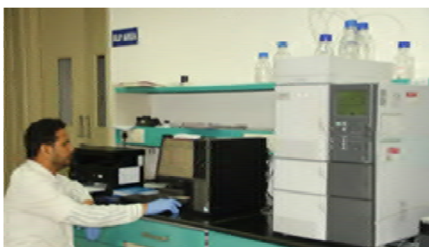
HPLC systems for carrying out tests and bioanalysis per the Indian Pharmacopoeia method 2.4.14 and other compendia in GLP-certified environment.
